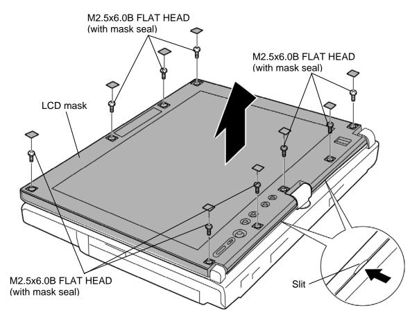
Figure 4-51 Removing the LCD mask
